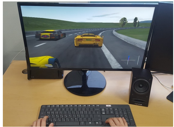
Fig. 7. The experimental setup that consists of a modified TORCS game, a keyboard controller, a speaker and a human driver.
